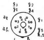
Base Connections Underside View of Base
