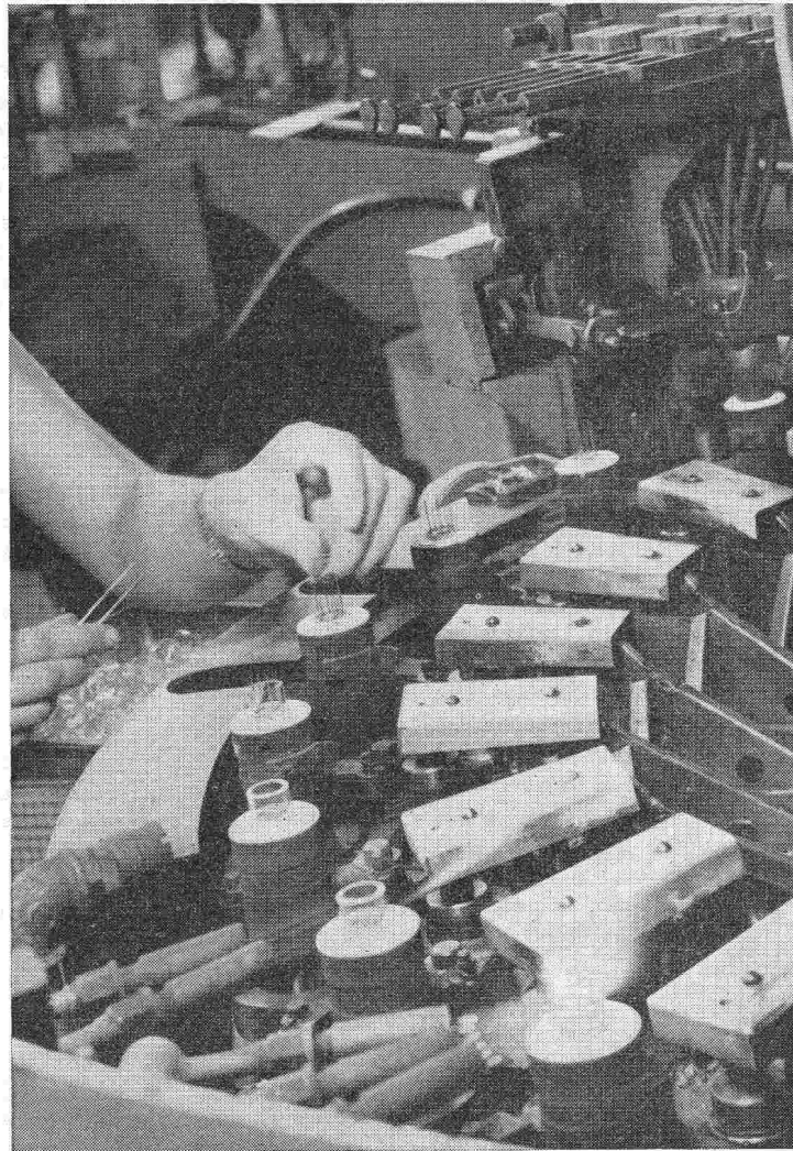
Fig. 1 — Making Miniature Valve Stems.
