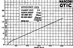
5 pin base. Standard I.H.C. triode connections.
