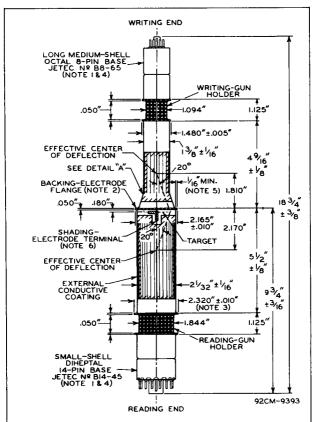
NOTE 1: THE PLANE THROUGH THE TUBE AXIS AND THE KEY OF THE DIHEPTAL BASE MAY VARY FROM THE PLANE THROUGH THE TUBE AXIS AND THE KEY OF THE OCTAL BASE BY AN ANGULAR TOLERANCE OF  $10^{\circ}$  MEASURED ABOUT THE TUBE AXIS. BOTH KEYS ARE ON THE SAME SIDE OF THE TUBE.
