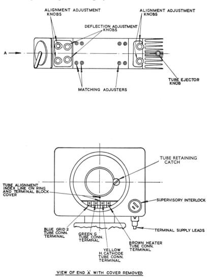
Fig. 10.—Diagram showing Operational Controls of WM110A
