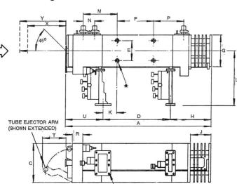
DIM. X (WITHDRAWAL DISTANCE OF TUBE WITH LATERAL MOVEMENT OF BASE) 12%" MIN. DIM. Y (WITHDRAWAL DISTANCE OF TUBE WITHOUT LATERAL MOVEMENT OF BASE) 15 MIN. \* DENOTES: 4-¼" UNC TAPPED HOLES BOTH SIDES
