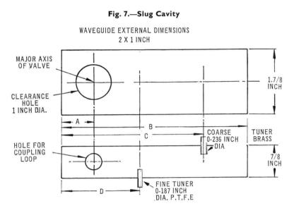
TRAVEL OF SLUGS JUST LESS THAN 7/8 INCH TO PREVENT CONTACT WITH OPPOSITE WAVEGUIDE WALL. NOTE: ALL DIMENSIONS SHOWN ARE INTERNAL DIMENSIONS.
