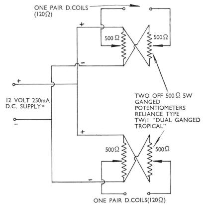
\*DENOTES:--THIS MAY BE OBTAINED FROM THE SOLENOID SUPPLY THROUGH A SUITABLE DROPPING RESISTOR
