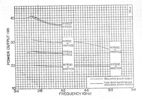
Fig. 1. Typical Power Output versus Frequency
