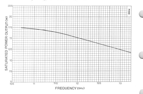
Fig. 1. Typical Saturated Output versus Frequency
