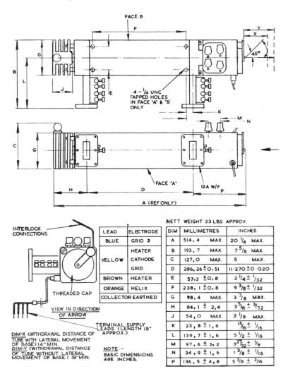
The collector is connected to the body of the mount and its earth path is via the mount body and the chassis to which the mount is attached. In some mounts a black lead is included in the cableform carrying the terminal supply leads: one end of this lead is connected to the body of the mount and the other may be earthed to provide an additional earth path.
