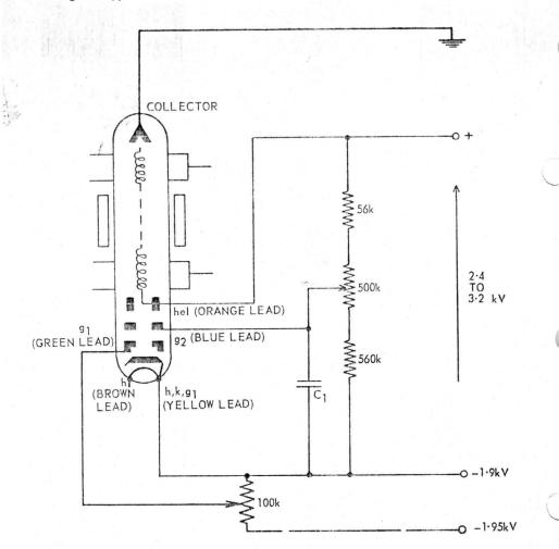
Fig. 7. Typical Cathode Current Control Circuit for W7/6F Series Tubes
