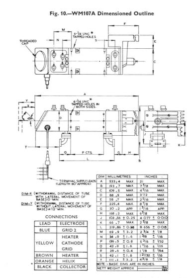
\*The collector is connected to the body of the mount and its earth path is via the mount body and the chassis to which the mount is attached. In some mounts a black lead is included in the cableform carrying the terminal supply leads: one end of this lead is connected to the body of the mount and the other may be earthed to provide an additional earth path.
