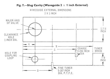
TRAVEL OF SLUGS JUST LESS THAN 7/8 INCH TO PREVENT CONTACT WITH OPPOSITE WAVEGUIDE WALL. NOTE: ALL DIMENSIONS SHOWN ARE INTERNAL DIMENSIONS.
