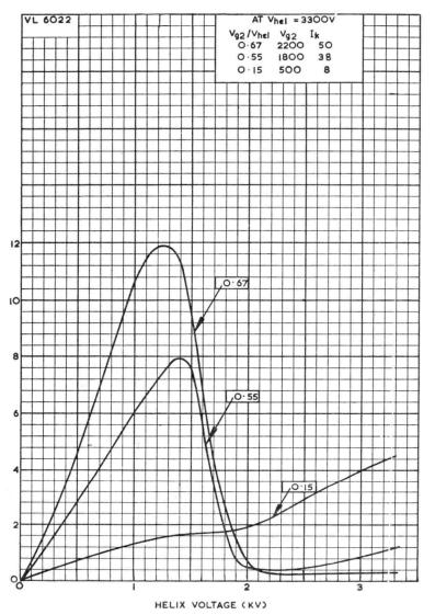
Fig. 7.-Typical Helix Current versus Helix Voltage
