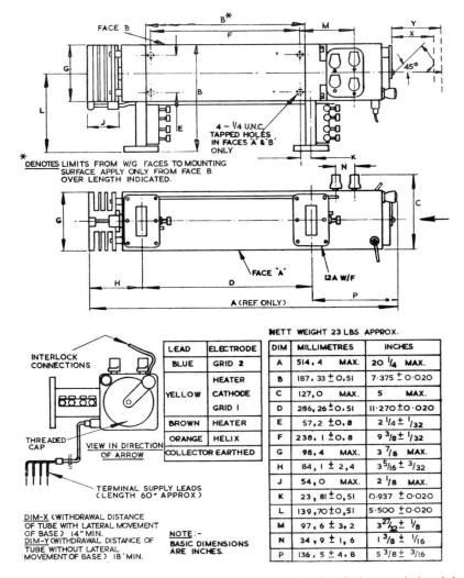
The collector is connected to the body of the mount and its earth path is via the mount body and the chassis to which the mount is attached. In some mounts a black lead is included in the cableform carrying the terminal supply leads: one end of this lead is connected to the body of the mount and the other may be earthed to provide an additional earth path.
