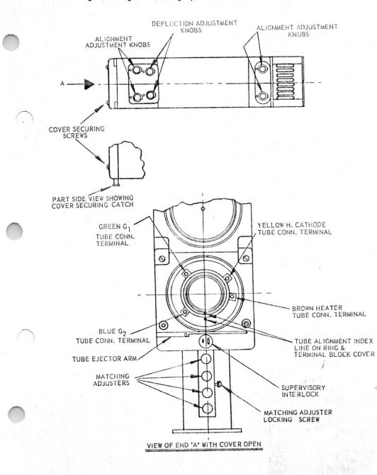
Fig. 12. Diagram Showing Operational Controls of WM111CA
