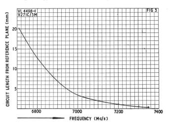
Fig. 3.-Typical Mechanical Tuning Characteristic.
