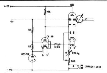
Fig. 2.—Circuit for stabilisation of V.M. oscillator tube current
