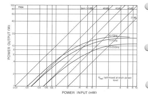
Fig. 5. Typical Power Output versus Power Input
