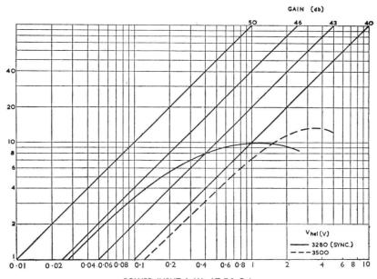
Fig. 2.-Typical Power Output versus Power Input at 7.8 Gc/s
