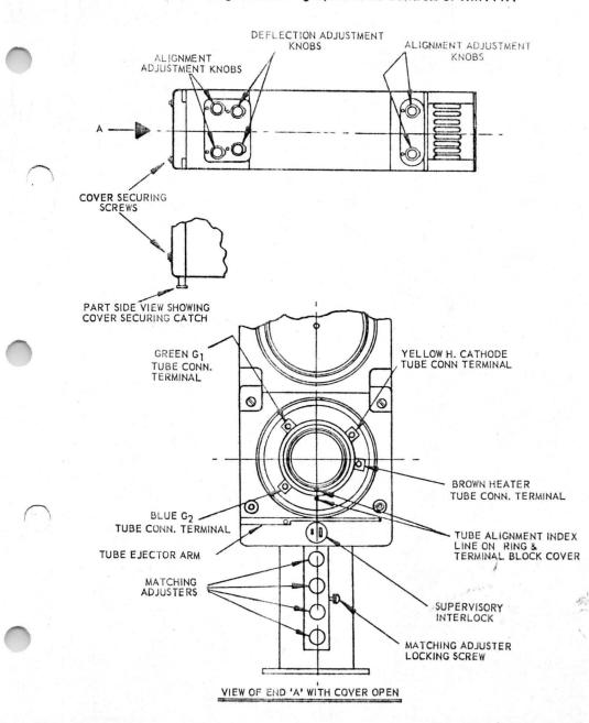
Fig. 10. Diagram Showing Operational Controls of WM111A
