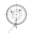
INDEX MARKS & PIN NO. 1 WILL NOT DEVIATE FROM A COMMON & BY MORE THAN 15° IN EITHER DIRECTION
