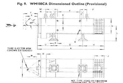
DIM-X (WITHDRAWAL DISTANCE OF TUBE WITH LATERAL MOVEMENT OF BASE) IO"MIN
