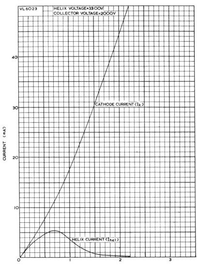
Fig. 8.-Typical Helix and Cathode Currents versus Grid 2 Voltage
