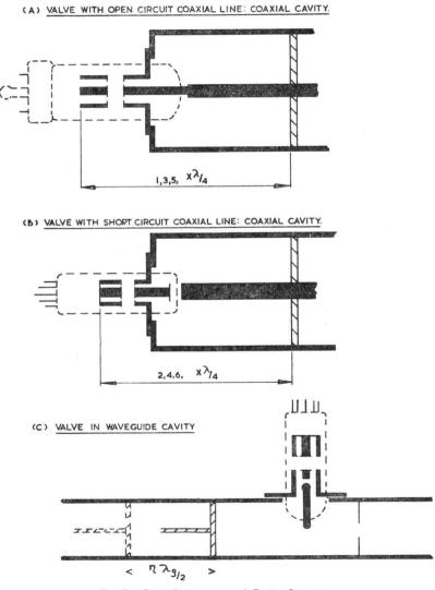
Fig. 3.—Basic Resonator and Cavity Structure
