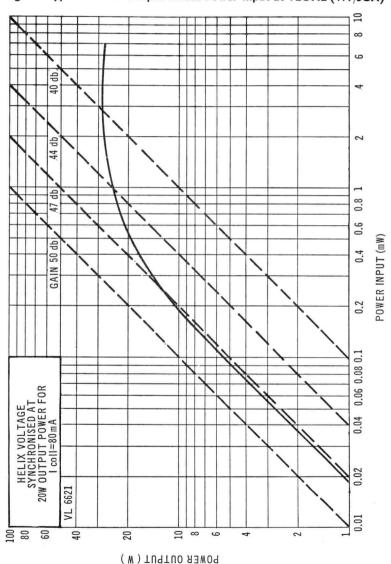
Fig. 3.-Typical Power Output versus Power Input at 4.2GHz (W7/5GA)
