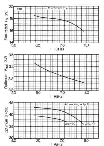
Fig. 1. Typical Output Power; Helix Voltage and Gain versus Frequency
