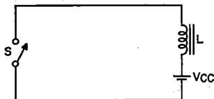
Fig. 85—Simplest form of deflection circuit.
