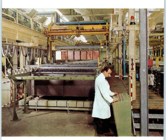
Part of the automatic plating installation showing process control console.
