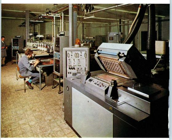
Forty-spindle automatic jig drilling machine (foreground).
