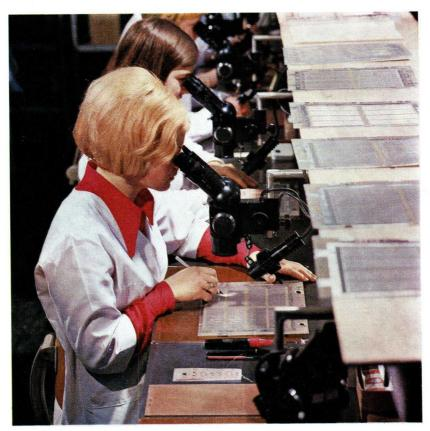
Inspection of conductor pattern.
