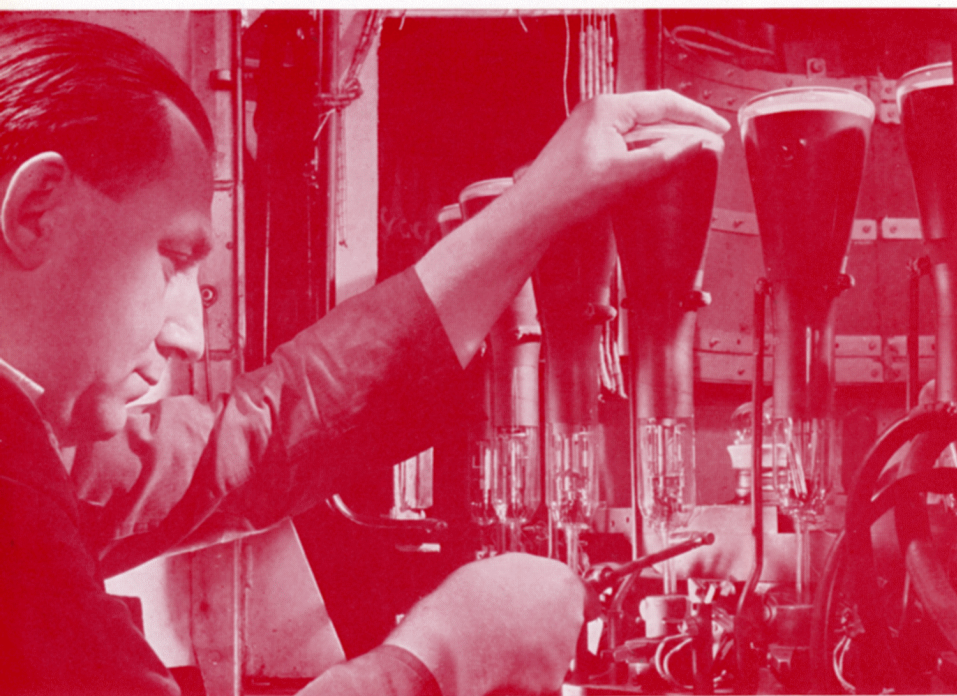
Pumping and sealing off is done on an intricate automatic machine. During the pumping process the tubes pass through several phases of normal and high-frequency heating to remove the last traces of gas.
