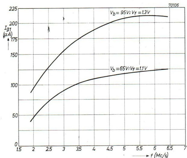
Fig. 105. Current I_{g1} flowing through the grid leak of the oscillator as a function of the frequency for the range S.W. 2 for nominal and reduced supply voltages.
