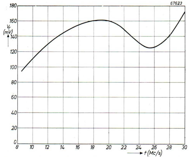
Fig. 6. Radiation voltage at the aerial terminals as a function of frequency.
