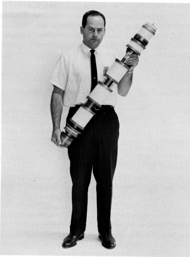
Figure 11—Recommended Method of Hand Carrying Eimac Klystrons.
